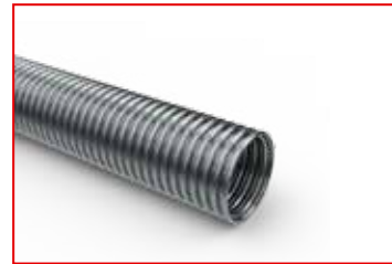
After the tube has been welded, corrugations are formed into the tube to make it flexible
