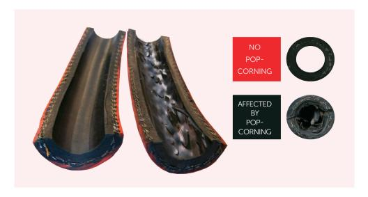
To overcome this 'popcorning'-effect, Goodall® developed a special, non-porous rubber compound for the inner tube of these two steam hoses. This tube is extruded and thus extremely smooth and non-porous.
